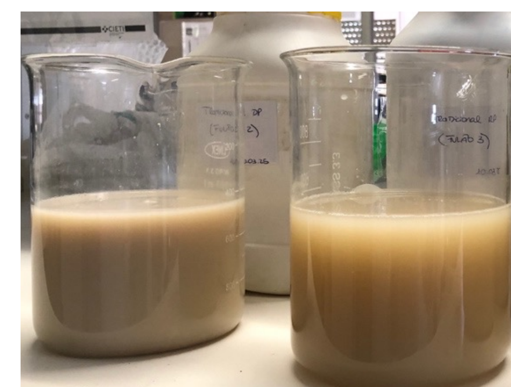
Figure 2 – Effluent of hair burning (left) and hair saving process (right)
