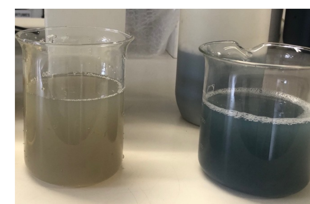
Figure 3 – Effluent of ecological chrome tanning (left) and traditional chrome tanning process (right)
